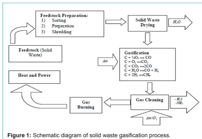
Figure 1: Schematic diagram of solid waste gasification process.
