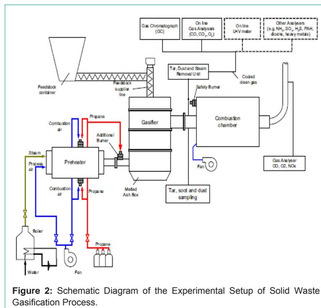
Figure 2: Schematic Diagram of the Experimental Setup of Solid Waste Gasification Process.
