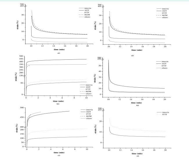
Figure 2: Creep and recovery curves: a1) creep @stress = 0.5 MPa, a2) recovery @stress = 0.5 MPa, b1) creep @stress = 1 MPa, b2) recovery @stress = 1 MPa, c1) creep @stress = 2 MPa, c2) recovery @stress = 2 MPa.
