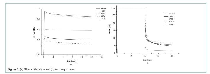
evidenced in the tensile test), whereas SIBS copolymers exhibited a visco-elastic behavior, undergoing increased deformation under the applied constant stress.
