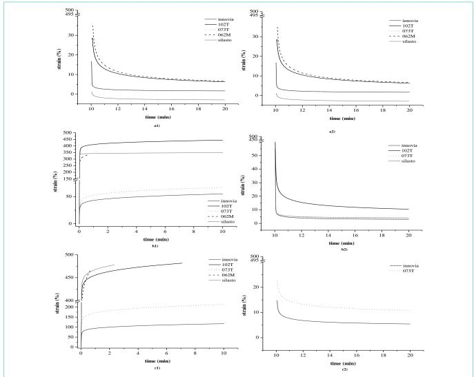
Figure 2: Creep and recovery curves: a1) creep @stress = 0.5 MPa, a2) recovery @stress = 0.5 MPa, b1) creep @stress = 1 MPa, b2) recovery @stress = 1 MPa, c1) creep @stress = 2 MPa, c2) recovery @stress = 2 MPa.
