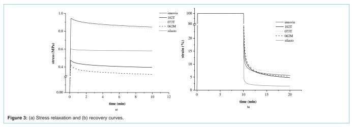
evidenced in the tensile test), whereas SIBS copolymers exhibited a visco-elastic behavior, undergoing increased deformation under the applied constant stress.
