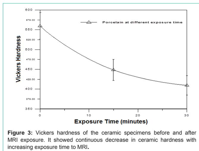
**Figure 3:** Vickers hardness of the ceramic specimens before and after MRI exposure. It showed continuous decrease in ceramic hardness with increasing exposure time to MRI.
