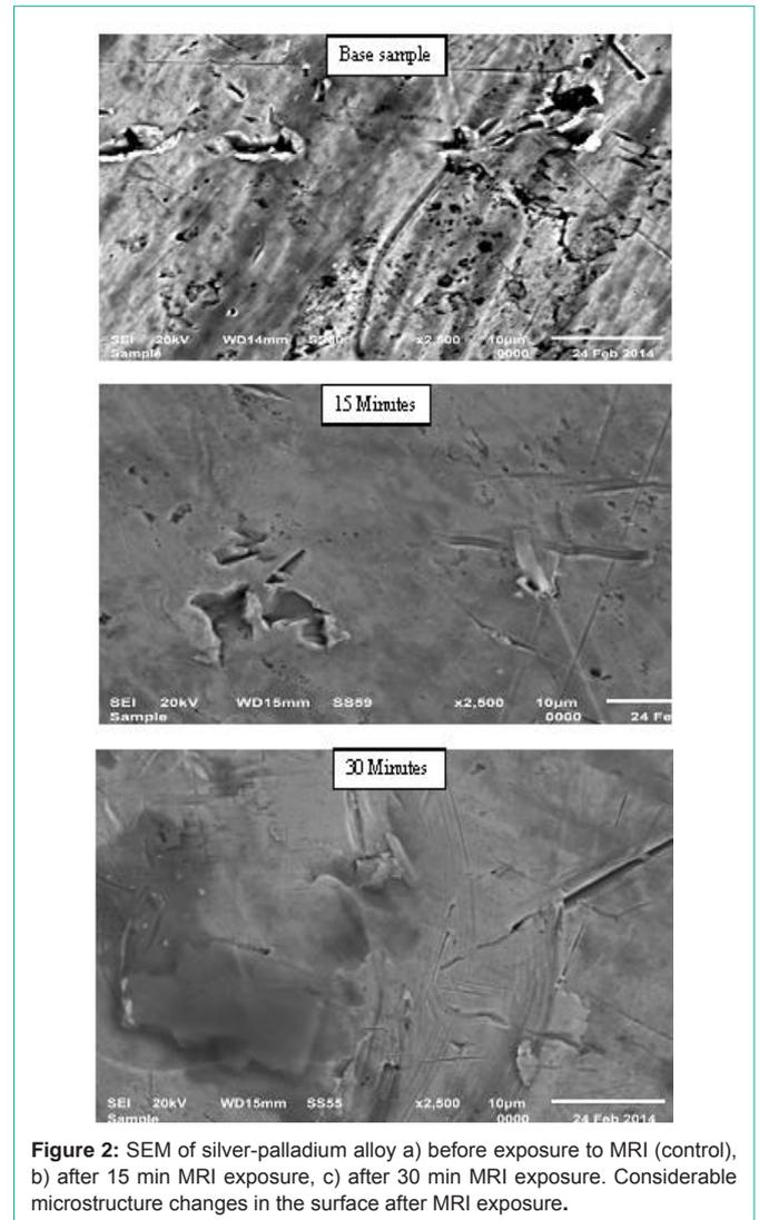
**Figure 2:** SEM of silver-palladium alloy a) before exposure to MRI (control), b) after 15 min MRI exposure, c) after 30 min MRI exposure. Considerable microstructure changes in the surface after MRI exposure.
