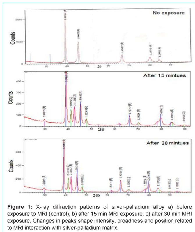
**Figure 1:** X-ray diffraction patterns of silver-palladium alloy a) before exposure to MRI (control), b) after 15 min MRI exposure, c) after 30 min MRI exposure. Changes in peaks shape intensity, broadness and position related to MRI interaction with silver-palladium matrix.
