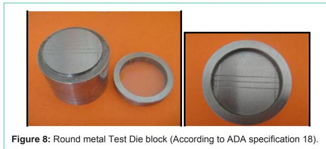
**Figure 8:** Round metal Test Die block (According to ADA specification 18).
