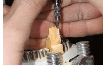
Figure 13: Parallelometer milling of individual dies.
