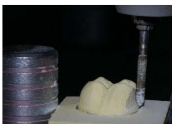
Figure 2: Parallelometer preparation of the cast.
