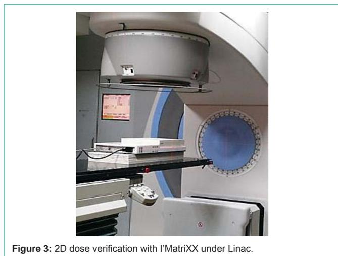
Figure 3: 2D dose verification with I'MatriXX under Linac.
