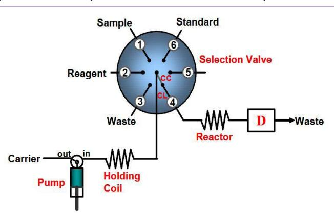
**Figure 3:** A typical SIA manifold. CC: central communication conduit, CL: central communication line, D: detector [10].
