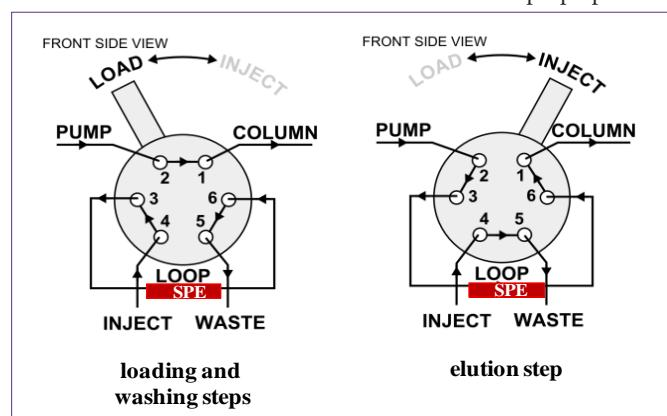
**Figure 8:** Schematic diagram of valves configuration for on-line SPE-HPLC system.
