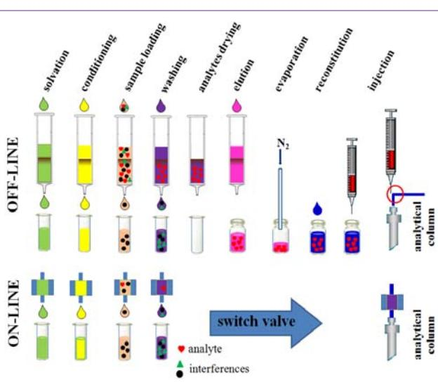
**Figure 2:** Schematic comparison of off-line versus on-line SPE coupled to HPLC.
