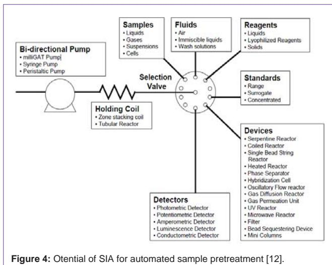
Figure 4: Potential of SIA for automated sample pretreatment [12].
