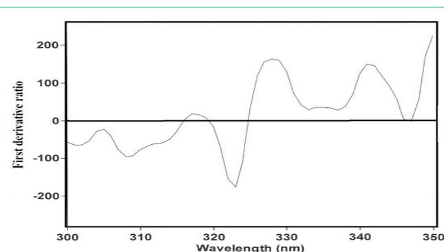
Figure 5: First derivative ratio spectra for 10 µg/mL of RN, using normalized spectrum of PL as a divisor.
