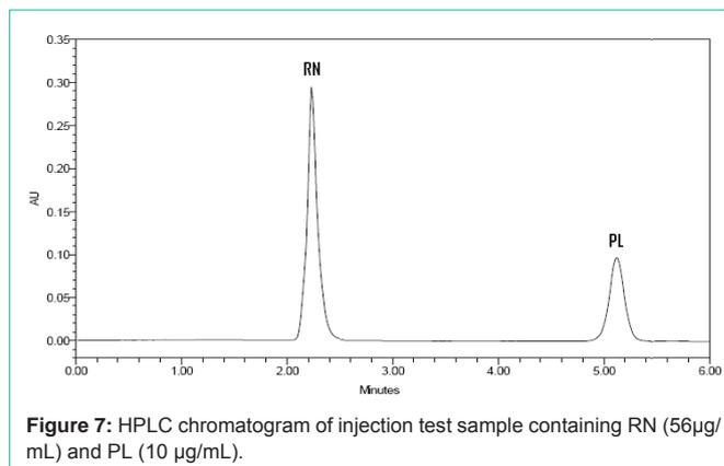
**Figure 7:** HPLC chromatogram of injection test sample containing RN (56 µg/mL) and PL (10 µg/mL).
