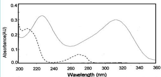
Figure 2: UV absorption spectra of 11.2 µg/mL RN (—) and 2 µg/mL PL (---) in water.
