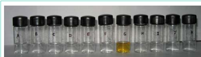
Figure 2: Photographs of mixture of 10 mM each of nitrite with various analytes (1.5 mL + 1.5 mL) in pH 2.06 KCl-HCl buffer solutions. AA = ascorbic acid; CA = catechol; CySH = cysteine; DA = dopamine; Glu = glucose; TURA = thiourea; UA = uric acid and URA = Urea.
