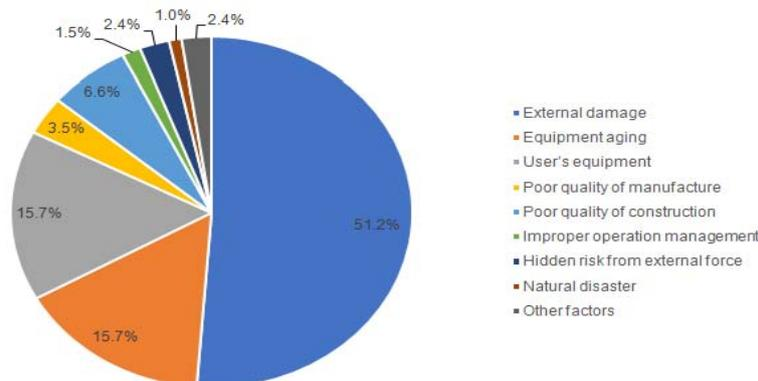
Figure 1: 2006 analysis of 10kV cable failure causes.
