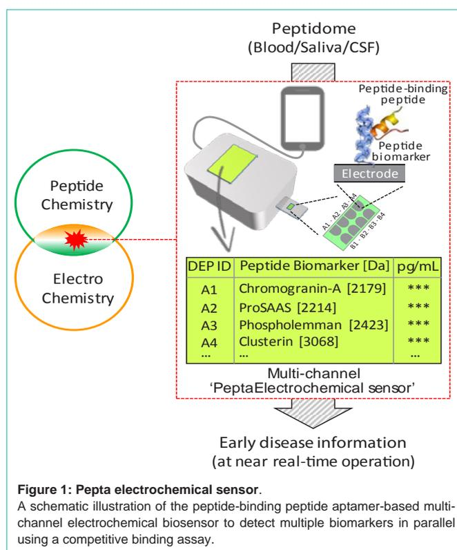
**Figure 1: Pepta electrochemical sensor.** A schematic illustration of the peptide-binding peptide aptamer-based multi-channel electrochemical biosensor to detect multiple biomarkers in parallel using a competitive binding assay.
