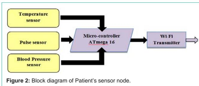
Figure 2: Block diagram of Patient's sensor node.
