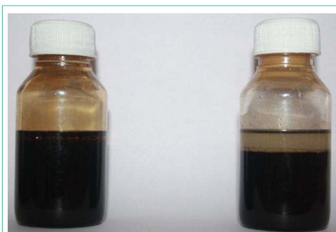
Figure 1: Visual appearance of (A) emulsions before treatment and (B) emulsified after treatment.
