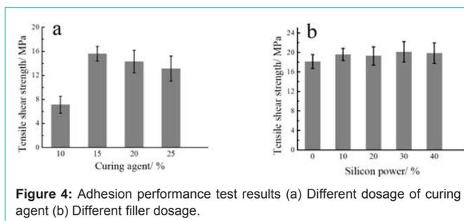
Figure 4: Adhesion performance test results (a) Different dosage of curing agent (b) Different filler dosage.
