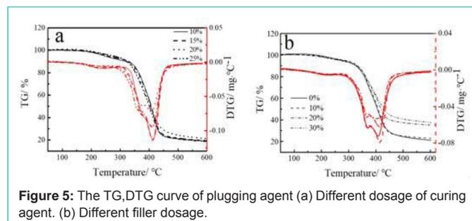
**Figure 5:** The TG,DTG curve of plugging agent (a) Different dosage of curing agent. (b) Different filler dosage.
