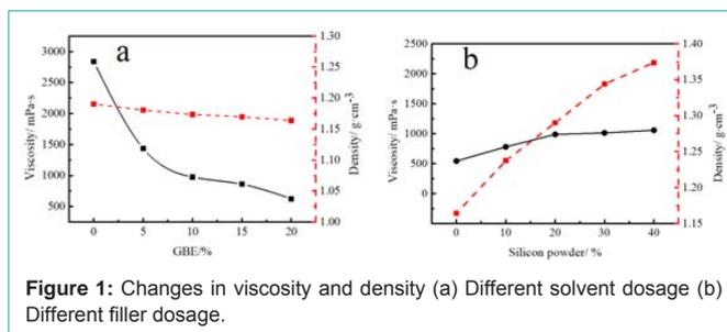
**Figure 1:** Changes in viscosity and density (a) Different solvent dosage (b) Different filler dosage.
