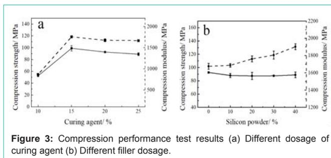
Figure 3: Compression performance test results (a) Different dosage of curing agent (b) Different filler dosage.
