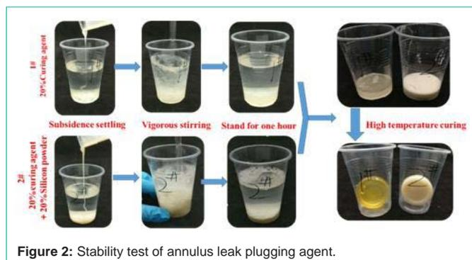
Figure 2: Stability test of annulus leak plugging agent.
