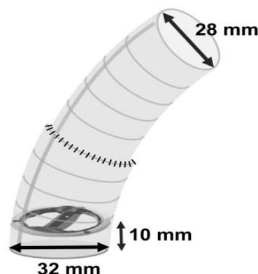
**Figure 2:** The composite graft was designed to suture the mechanical valve with a 10-mm margin from the end of the proximal side. The distal side of the graft was connected to another one (32–28 mm) to adjust the diameter of the native aorta.
