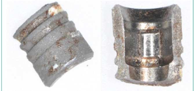
Figure 6: Only one part of the fractured implant (a) was still present when the patient reported to our clinic consisting of approximately 50% of the circumference of the implant abutment connection (b).
