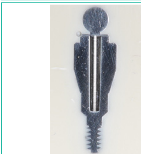
Figure 13: Cross-sectional view of a prototype flexible attachment system (Reflex, Hader Solutions & Distribution) with a ball mounted on a centrally positioned beam allowing for lateral movement while maintaining vertical dimensions.
