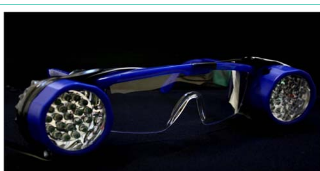
Figure 2: Binocular with auxiliary standard LED D65 light source.
