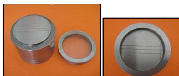
**Figure 8:** Round metal Test Die block (According to ADA specification 18).
