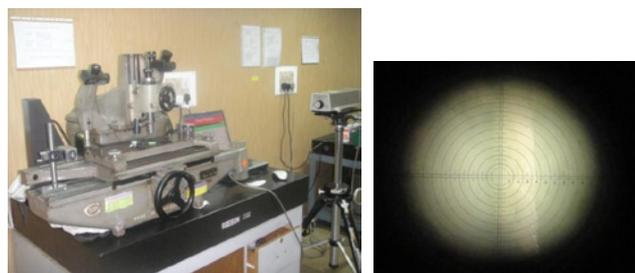
Figure 10: Measuring the linear scores between the reference lines obtained from the Test Die under a Universal Measuring Microscope.
