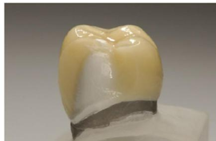
**Figure 4:** Cohesive fracture of a specimen from layering technique (Beuer).
