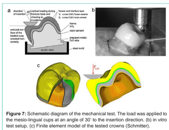
**Figure 7:** Schematic diagram of the mechanical test. The load was applied to the mesio-lingual cups at an angle of 30° to the insertion direction. (b) in vitro test setup. (c) Finite element model of the tested crowns (Schmitter).
