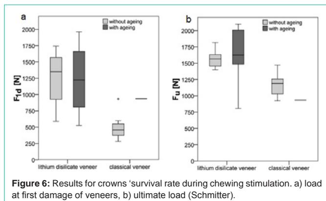
**Figure 6:** Results for crowns 'survival rate during chewing stimulation. a) load at first damage of veneers, b) ultimate load (Schmitter).
