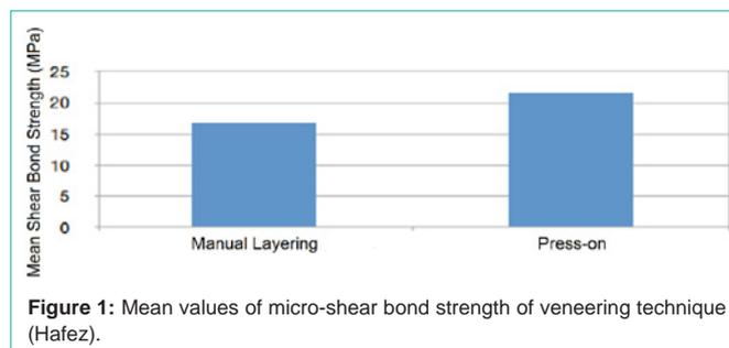
Figure 1: Mean values of micro-shear bond strength of veneering technique (Hafez).
