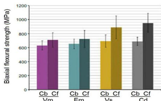
**Figure 10:** The effect of veneering ceramic types on the fracture strength (Tangatchatham).
