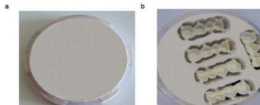
**Figure 11:** CAD/CAM veneer blanks, a) before and b) after milling.
