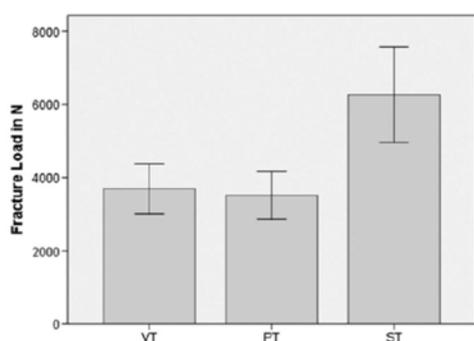
**Figure 3:** Fracture load of layered (VT), heat-pressed-on (PT), and CAD/CAM (ST) veneering on zirconia frameworks (Beuer).
