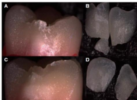
**Figure 2:** Stereomicroscope images of fractured zirconia frameworks, (A) lingual view of pressed veneered zirconia and (B) fractured segments (cohesive within ceramic), (C) lingual view of layered veneered zirconia and (D) fractured parts (adhesive) (Turk).
