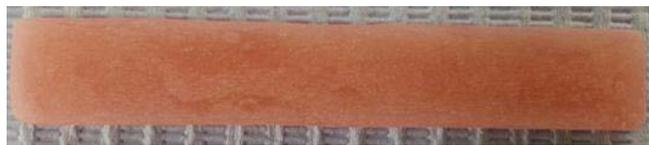
Figure 1: The prepared specimen for flexural properties testing.
