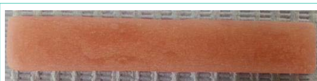
Figure 1: The prepared specimen for flexural properties testing.
