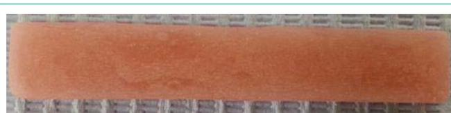
**Figure 1:** The prepared specimen for flexural properties testing.
