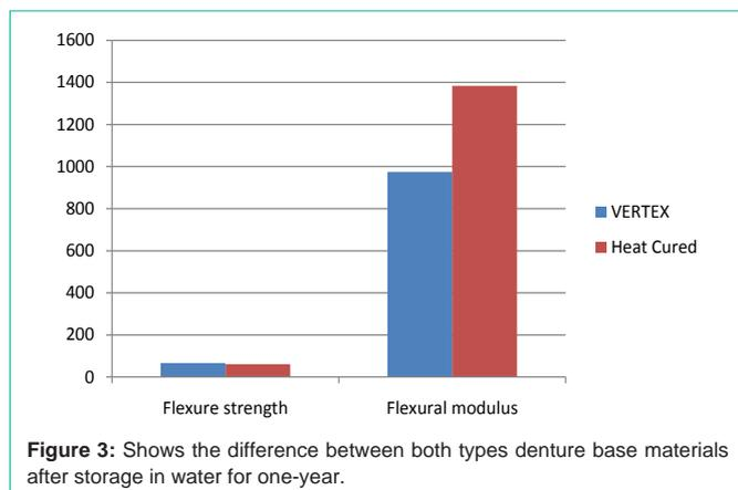
using Instron Universal Testing Machine (Instron, USA.) with load cell 500 N Bluehill Lite software at cross head speed 1mm/min. The maximum load for fracture was recorded in (N) and the deflection of the specimens at fracture was recorded in mm. For calculating the flexural strength in MPa, the following formula was used:  $\text{Stress} = 3 \times \text{Load} \times \text{Length} / (2 \times \text{Width} \times \text{Thickness}^2)$  [16,17]
