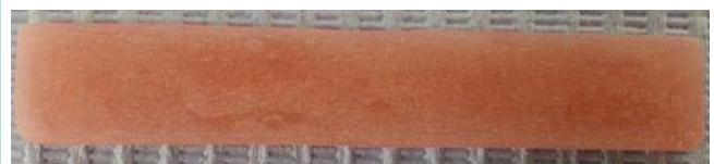
Figure 1: The prepared specimen for flexural properties testing.
