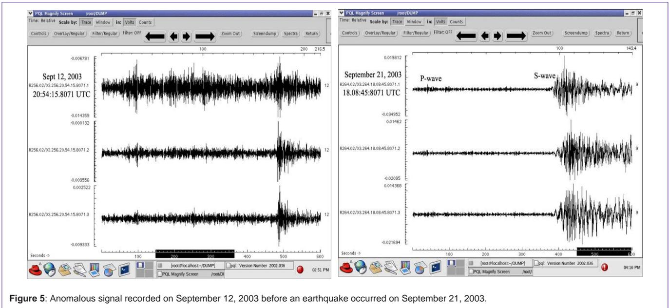
Figure 5: Anomalous signal recorded on September 12, 2003 before an earthquake occurred on September 21, 2003.
