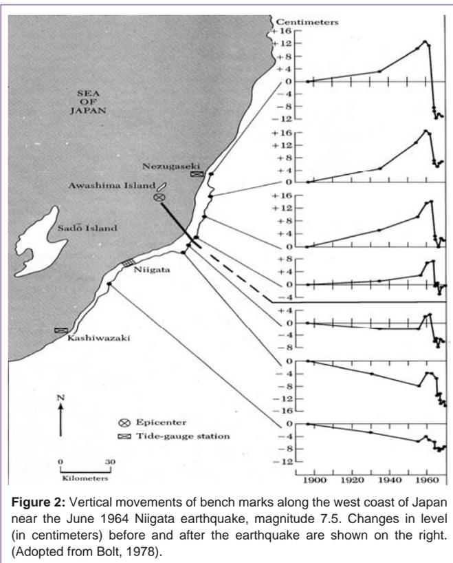
Figure 2: Vertical movements of bench marks along the west coast of Japan near the June 1964 Niigata earthquake, magnitude 7.5. Changes in level (in centimeters) before and after the earthquake are shown on the right. (Adopted from Bolt, 1978).
