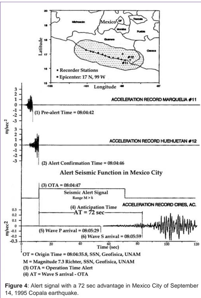
**Figure 4:** Alert signal with a 72 sec advantage in Mexico City of September 14, 1995 Copala earthquake.
