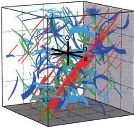
**Figure 7:** Progress of a large dislocation avalanche in [010] symmetrical multiple slip. Several geometrically separated dislocations become unpinned during the same event, which demonstrates the importance of long-range elastic interactions in strain burst initiation. The avalanche has a strongly anisotropic shape with more than 60% of the deformation occurring on one of the four equivalent sets of slip planes.
