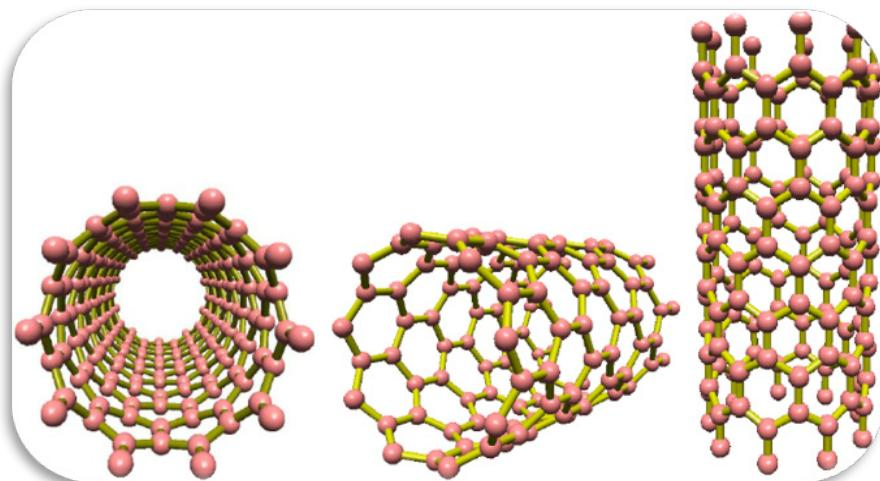
**Figure 5:** Three different structures of SWCNTs.
