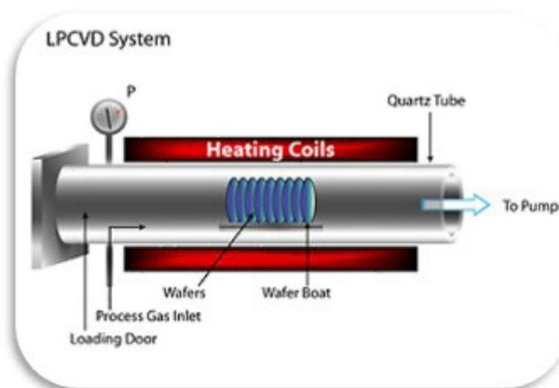
**Figure 10:** Schematic diagram of CVD.
