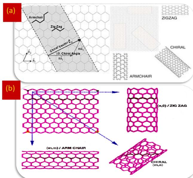
**Figure 4:** (a) Various parameters of CNTs (b) Helicity of graphene sheet.
