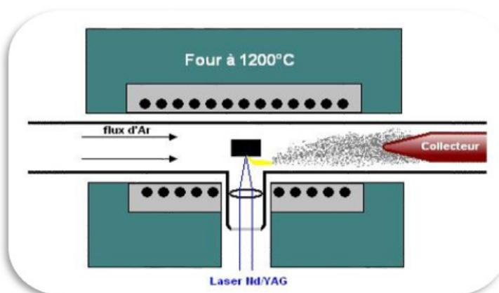
Figure 8: Laser ablation technique.
