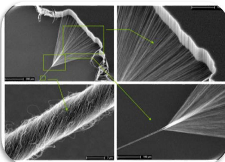
**Figure 19:** Threads like CNTs to reinforce in textiles.
