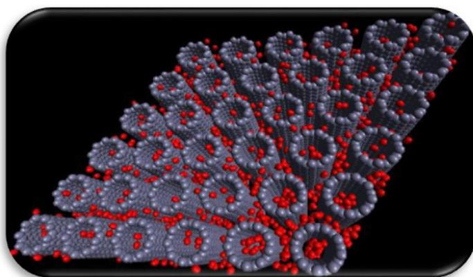
**Figure 18:** Hydrogen gas adsorbed in CNTs.
