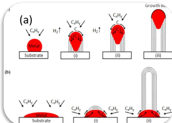
**Figure 12:** Growth mechanisms of CNTs: (a) Tip-Growth (b) Base Growth.
