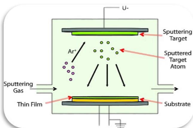
Figure 9: RF-sputtering technique.
