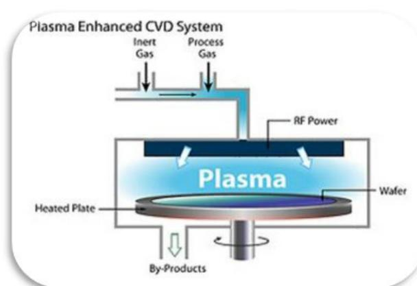
**Figure 11:** Schematic of PECVD technique.
