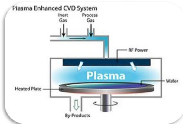
**Figure 11:** Schematic of PECVD technique.
