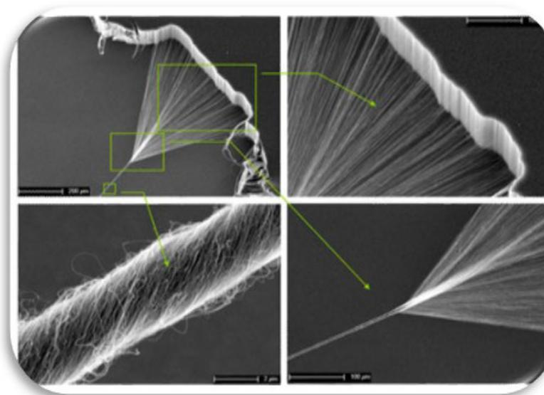
**Figure 19:** Threads like CNTs to reinforce in textiles.
