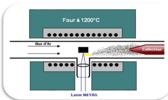
Figure 8: Laser ablation technique.
