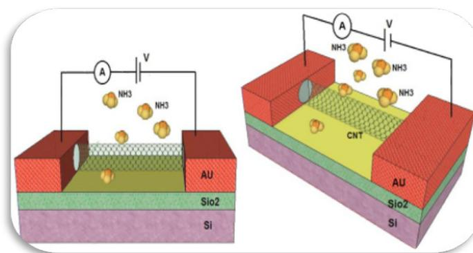
Figure 14: Schematic of CNT based Chemical sensor.
