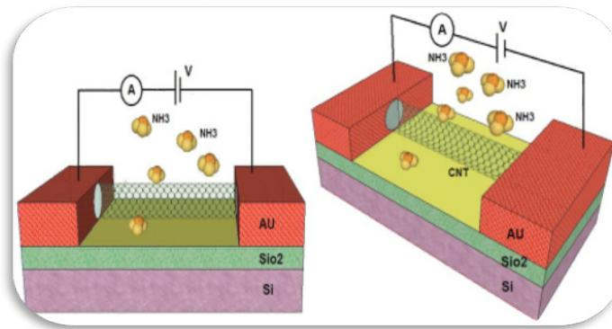
**Figure 14:** Schematic of CNT based Chemical sensor.
