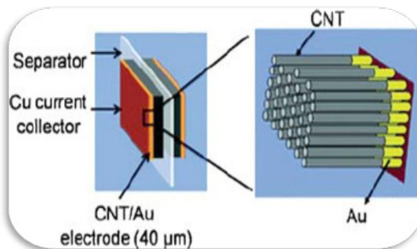
**Figure 17:** A super capacitor device with CNT/Au as the electrodes.
