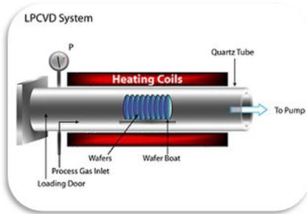
**Figure 10:** Schematic diagram of CVD.
