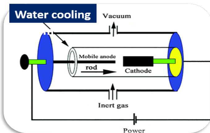
Figure 7: Arc discharge setup for CNT Growth.
