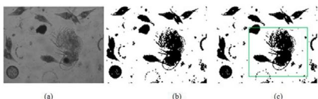
Figure 2: Image analysis process for >50  $\mu\text{m}$  species. (a) Original CCD image (b) Converting into binary image (c) Selecting an object.
