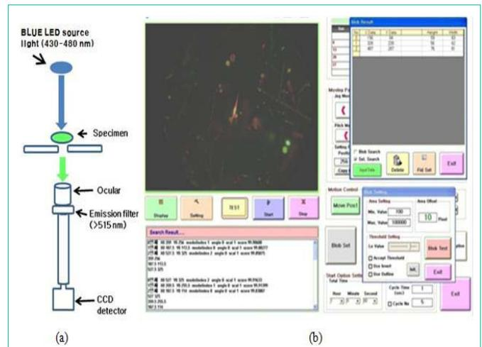
Figure 4: The counting system developed for 10~50 μm species. (a) Schematic of the counting apparatus (b) Screen shot of the counting system.
