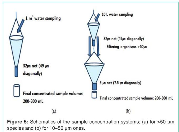
Figure 5: Schematics of the sample concentration systems; (a) for >50 μm species and (b) for 10~50 μm ones.
