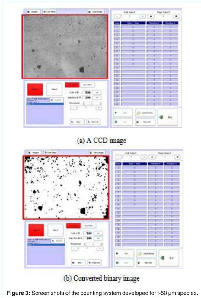
Figure 3: Screen shots of the counting system developed for >50 µm species.
