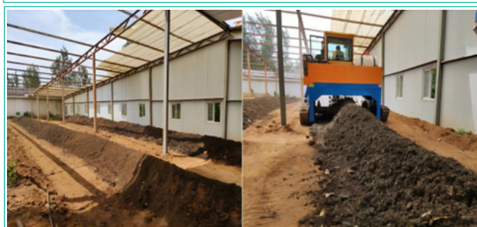
Figure 5: Strip composting diagram of a sanitation company in Qingdao, with kitchen and garden waste co-composting on site.
