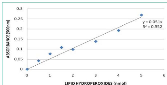
**Figure 6a:** Standard curve for Lipid Hydro Peroxides (LPO) assay where y-axis represents absorbance at 500nm whereas x-axis represents the concentrations of reference standard (nmol).
