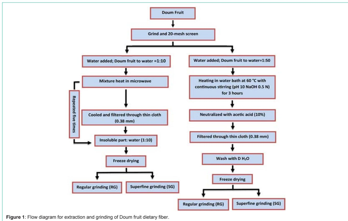
Figure 1: Flow diagram for extraction and grinding of Doum fruit dietary fiber.
