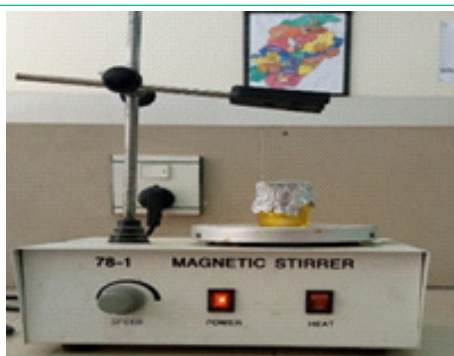
Figure 4: The image shows a magnetic stirrer with heating — a common lab device used to mix and gently heat solutions uniformly.
