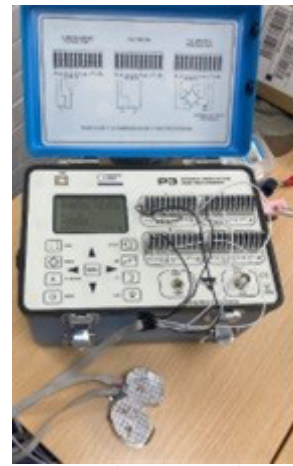
Figure 21: Sensor connected to strain indicator.
