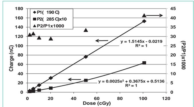
**Figure 3:** The TLD dose response of peaks P1 and P2 to 6 MV photons illustrating the sensitivity differences between the two peaks. P2 exhibits supralinearity above about 30 cGy.
