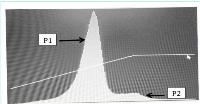
**Figure 1:** Glow curve obtained for a TLD irradiated to an absorbed dose of 20 cGy in a clinical proton beam illustrating the two temperature peaks. P1 represents the lower temperature peak and P2 is the higher temperature peak.
