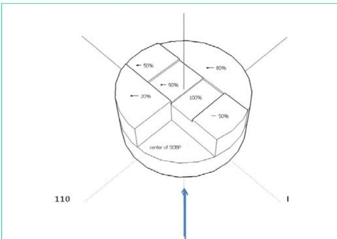
**Figure 2:** Schematic diagram of the cylindrical phantom used for measurements along the proton beam showing the location of the TLD700 detectors at the various depths. The arrow indicates the direction of the incident proton beam.
