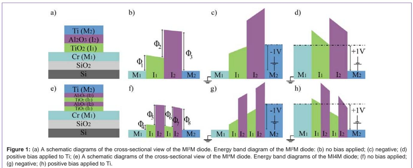
1c and Figure 1d under the same bias conditions, it can be concluded that the difference in the energy band diagram leading to asymmetry in MIM diodes. The same effect was also observed for the MI<sup>4</sup>M diode as it can be seen from Figure 1g and Figure 1h.
