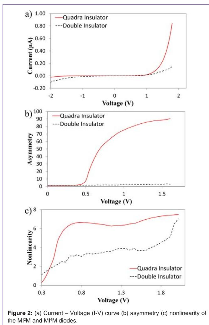
**Figure 2:** (a) Current – Voltage (I-V) curve (b) asymmetry (c) nonlinearity of the MI<sup>2</sup>M and MI<sup>4</sup>M diodes.
