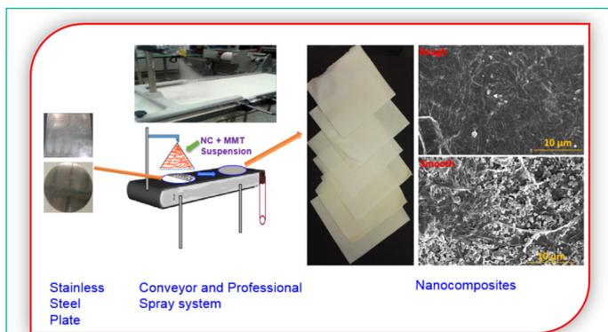
**Figure 1:** An experimental set up for spraying of nanocellulose suspension with MMT.
