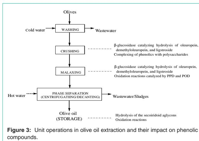
**Figure 3:** Unit operations in olive oil extraction and their impact on phenolic compounds.
