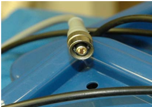
Figure 5: To evaluate the light cord, disconnect it from the light source and hold this end towards the ceiling lights. Now look on end at the scope connection and one can see small black areas representing broken fibers. If more than 30% of the fibers are broken, a new cord should be requested.
