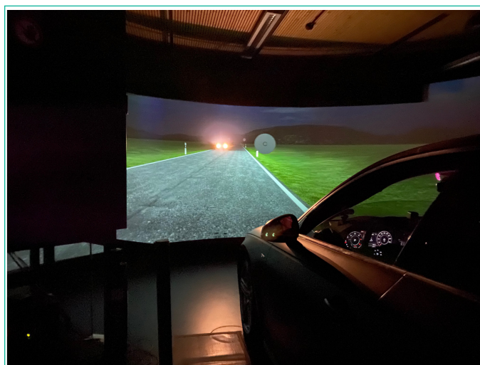
Figure 1: Photograph of the Aalen Night-Time Driving Simulator: The housing of one of the two LED planetarium projectors is visible at the left upper corner, the car (AUDI A4, right lower half of the image) is facing the hemi-cylindrical projection screen, with a LANDOLT C on the right side of the straight rural road. Two cable robots with moving LED glare sources simulate the headlights of the virtual vehicle in the oncoming lane.
