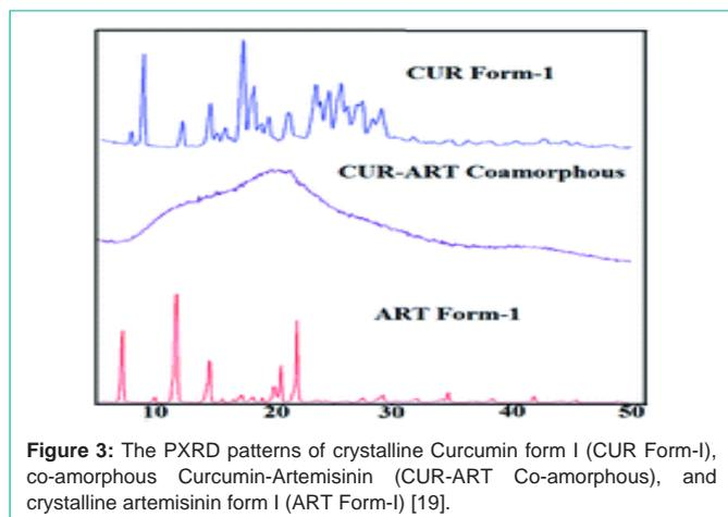
**Figure 3:** The PXRD patterns of crystalline Curcumin form I (CUR Form-I), co-amorphous Curcumin-Artemisinin (CUR-ART Co-amorphous), and crystalline artemisinin form I (ART Form-I) [19].
