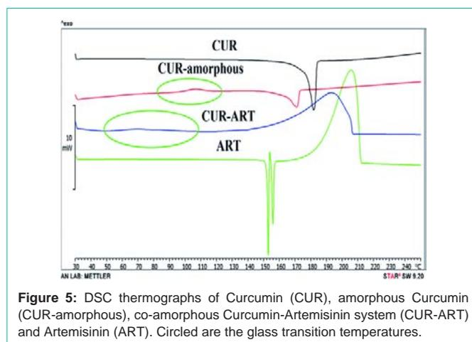
**Figure 5:** DSC thermographs of Curcumin (CUR), amorphous Curcumin (CUR-amorphous), co-amorphous Curcumin-Artemisinin system (CUR-ART) and Artemisinin (ART). Circled are the glass transition temperatures.
