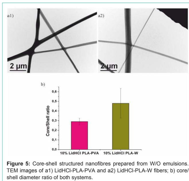
**Figure 5:** Core-shell structured nanofibres prepared from W/O emulsions. TEM images of a1) LidHCl-PLA-PVA and a2) LidHCl-PLA-W fibers; b) core/shell diameter ratio of both systems.
