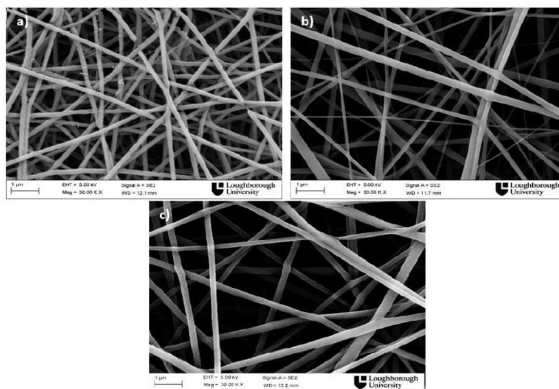
**Figure 3:** SEM images of electrospun emulsions loaded with 10% of drug. a) control LidHCl-PLA blend sample showing the drug located on the fiber surface and between them, b) LidHCl-PLA-PVA fibers and c) LidHCl-PLA-W fibers.
