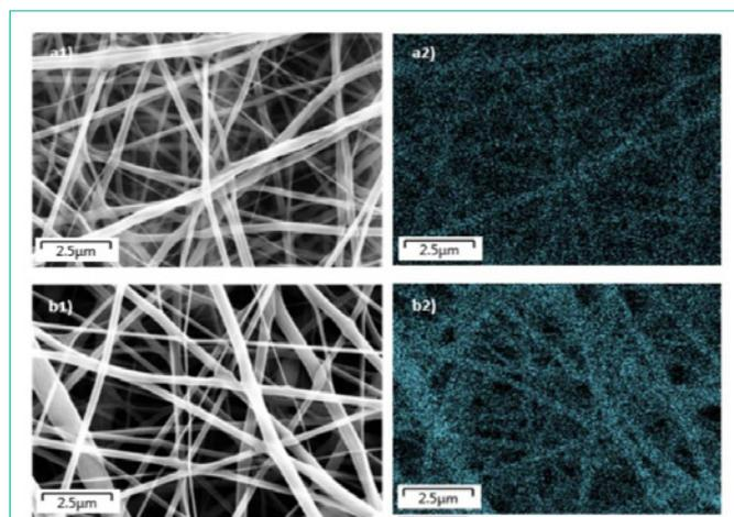
**Figure 4:** Micrographs and EDS maps of nitrogen. Pattern match between emulsion electrospun fibers and N distribution confirming the presence of the drug in LidHCl-PLA-PVA fibers (a1, a2) and LidHCl-PLA-W fibers (b1, b2), respectively.
