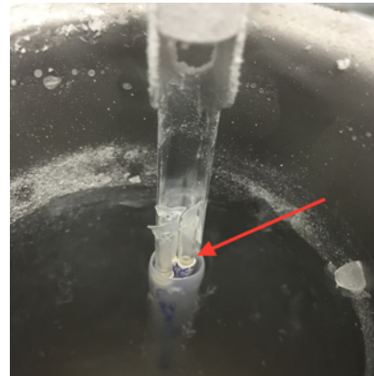
Figure 2: Upon inspecting a group of hybrid –vitrified straws transferred to our lab in the spring of 2016, we observed LN 2 present in the inner lumen of all seals (see arrow), which appeared to possess closed seals. The originating lab failed to provide accurate procedural paper work mentioning the latter potential flaw in their ‘cut-straw, rapid plunge, vapor sealed-closed straw system’, and how to safely warm incompletely sealed straws.
