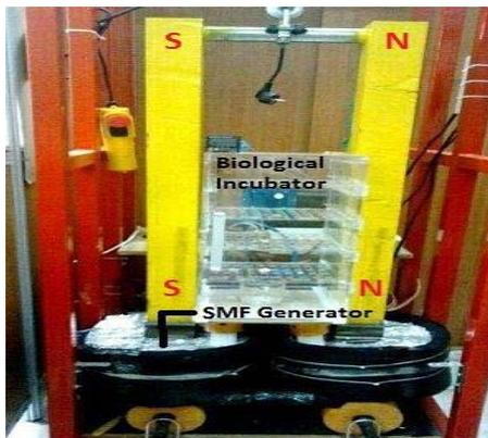
**Figure 1:** SMF generator equipped with a biological Incubator for providing standard cell culture conditions.
