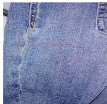
Figure 11: Spandex breakage in the sewing line.
