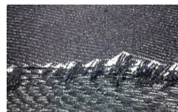
Figure 12: Spandex breakage due to cutting of fabric.
