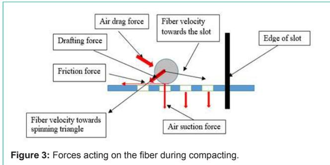
Figure 3: Forces acting on the fiber during compacting.
