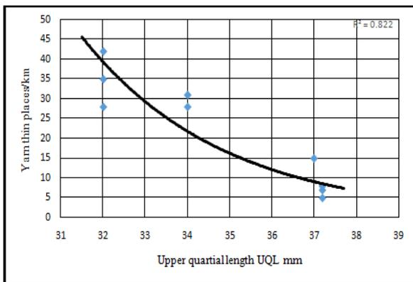
Figure 7: Number of yarn thin places/km versus UQL mm.
