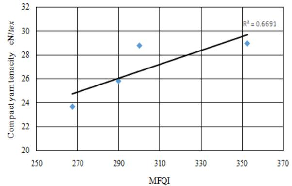
Figure 9: Compact yarn strength versus MFQI.
