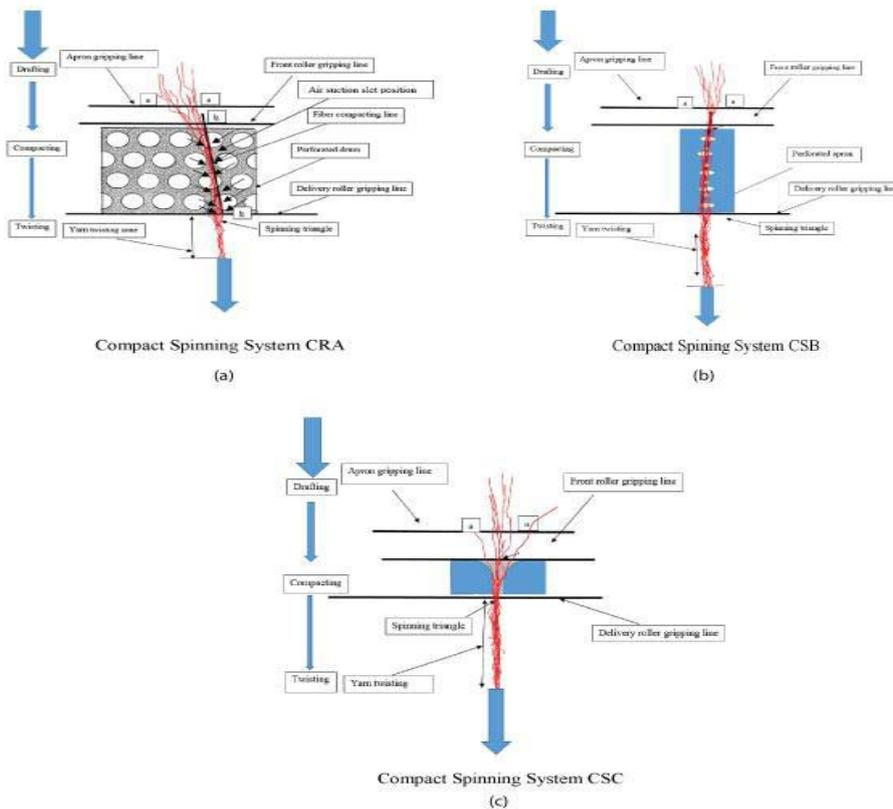
Figure 2 (a, b, c): Principles of Compact Spinning Systems.
