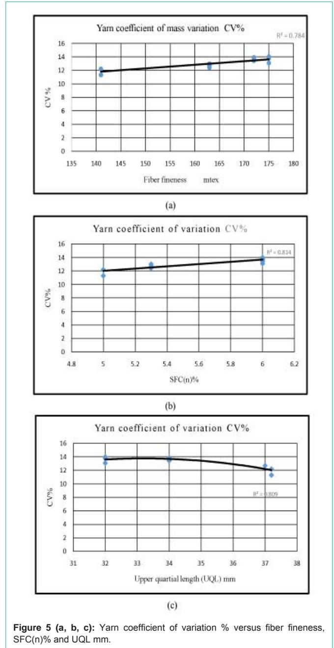
Figure 5 (a, b, c): Yarn coefficient of variation % versus fiber fineness, SFC(n)% and UQL mm.
