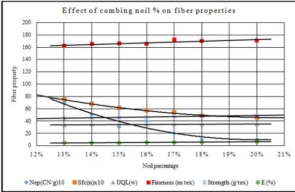
Figure 10: Fiber properties versus the noil percentage.
