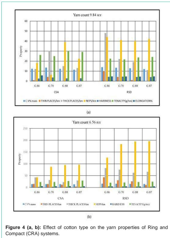
Figure 4 (a, b): Effect of cotton type on the yarn properties of Ring and Compact (CRA) systems.
