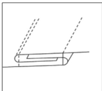
Figure 3: Lapped seam.
