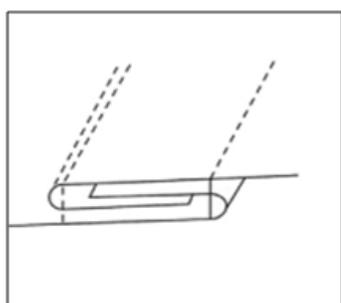
Figure 3: Lapped seam.
