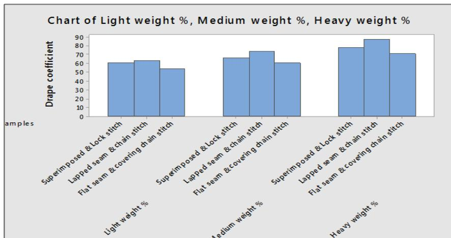
Figure 12: Drape coefficient of different seamed fabric with stitches.
