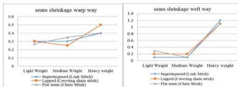
Figure 11: Seam shrinkage in warp and weft way direction.
