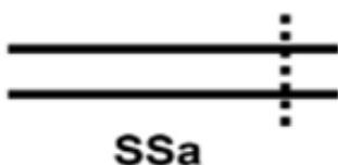
Figure 2: Superimposed seam.
