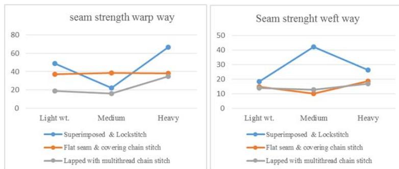
Figure 9: Seam strength in warp and weft way.
