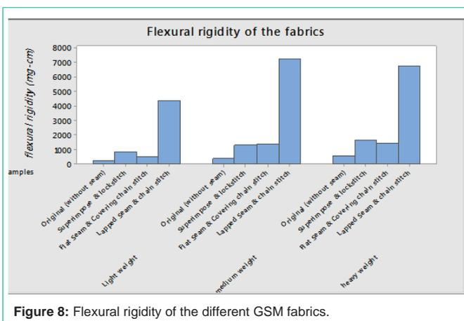
Figure 8: Flexural rigidity of the different GSM fabrics.
