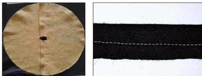
Figure 1: Sample preparation for drupe coefficient and stiffness.
