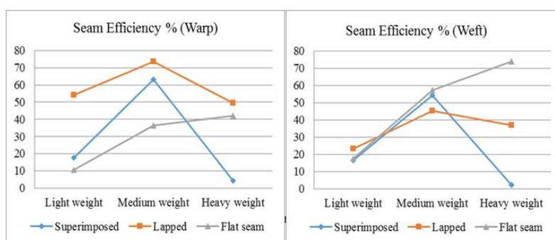
Figure 10: Seam efficiency in warp and weft direction.
