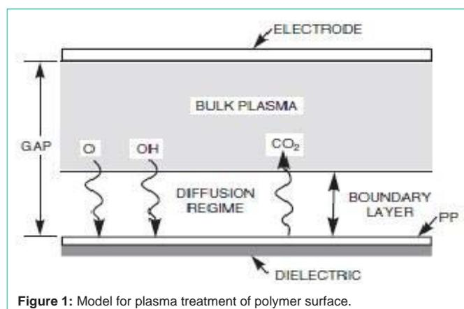
Figure 1: Model for plasma treatment of polymer surface.
