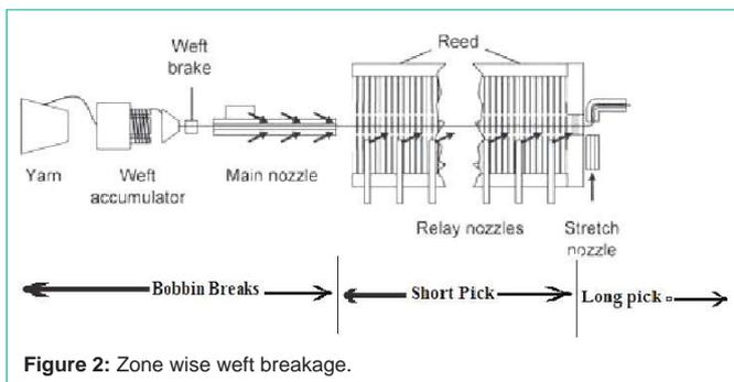
**Figure 2:** Zone wise weft breakage.
