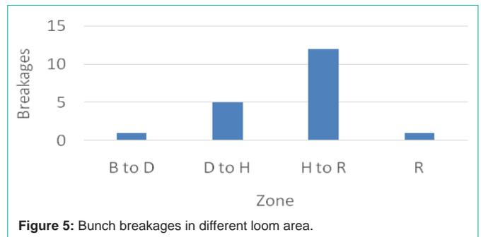
**Figure 5:** Bunch breakages in different loom area.
