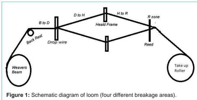
**Figure 1:** Schematic diagram of loom (four different breakage areas).
