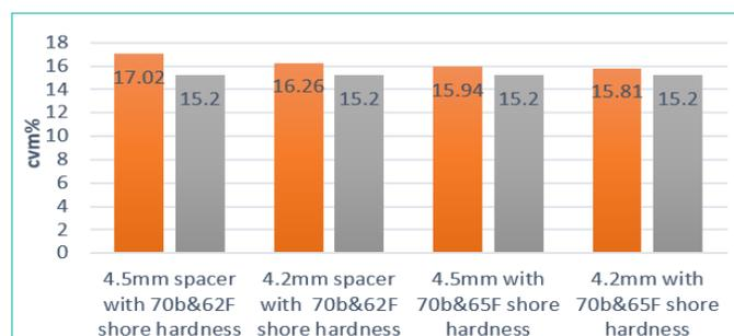
**Figure 2:** Effect of 4.5 & 4.2 mm spacer size with 62 & 65 degree of shore hardness front top roller on yarn coefficient.
