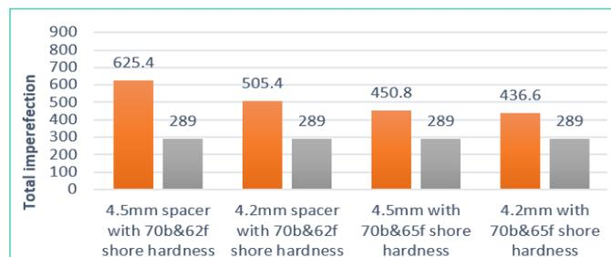
**Figure 3:** The effect of 4.5 & 4.2 mm spacer size combination with 62 & 65 degree of shore hardness front top roller.
