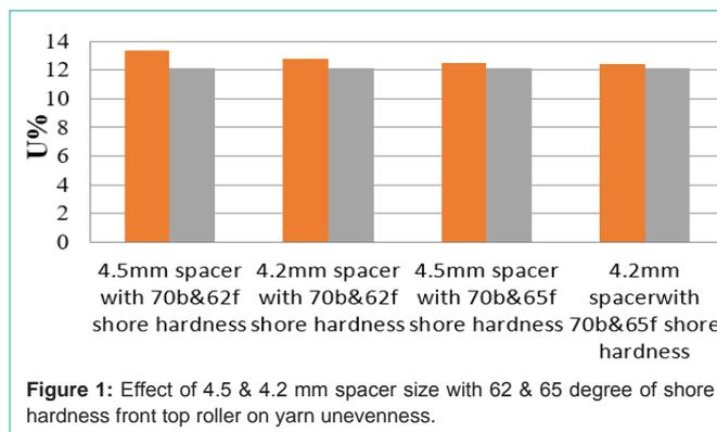
hardness on the yarn unevenness is plotted in (Figure 1). The spacer of 4.2mm with 62 degrees of shore hardness gives the best even yarn with a low u% of 35.5Nm. In the case of smaller spacer sizes there is better control of short fibers. Evenness is improved by closing down the apron spacing.
