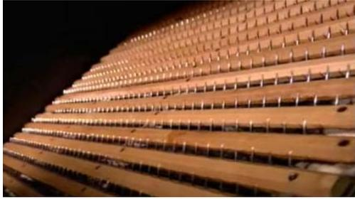
Figure 4: Conveyor with protruding spikes for carding process.
