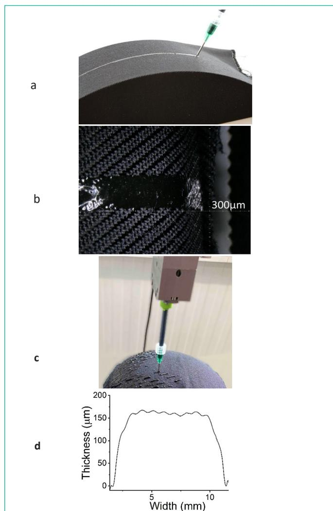
**Figure 6:** a) Robot-assisted dispensing process of a line on an elliptic curved gabardine textile using the Vipro head dispensing unit integrated on a UR 10 robot; b) microscopic view of the dispensed HAPTIC® ink on curved surfaces. c) Robot-assisted dispensing of TPU test structures on spherical knitted fleece fabric with its shape retaining behavior profilometry measurement of dispensed HAPTIC® onto gabardine textile with an average layer thickness of 165  $\mu\text{m}$  (d).
