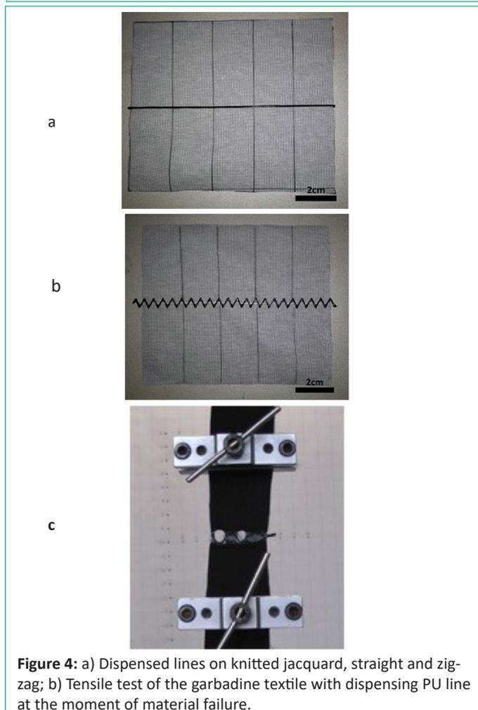
**Figure 4:** a) Dispensed lines on knitted jacquard, straight and zig-zag; b) Tensile test of the gabardine textile with dispensing PU line at the moment of material failure.
