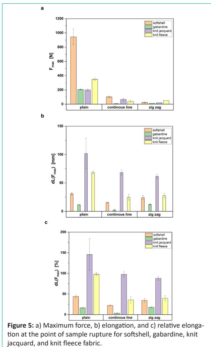
**Figure 5:** a) Maximum force, b) elongation, and c) relative elongation at the point of sample rupture for softshell, gabardine, knit jacquard, and knit fleece fabric.
