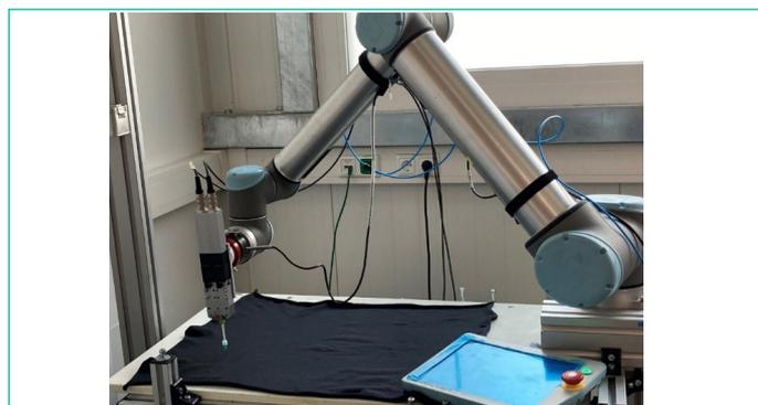
Figure 2: Robot-assisted dispensing setup for dispensing the waterborne HAPTIC® ink formulation on a flat gabardine textile.
