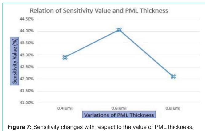
Figure 7: Sensitivity changes with respect to the value of PML thickness.
