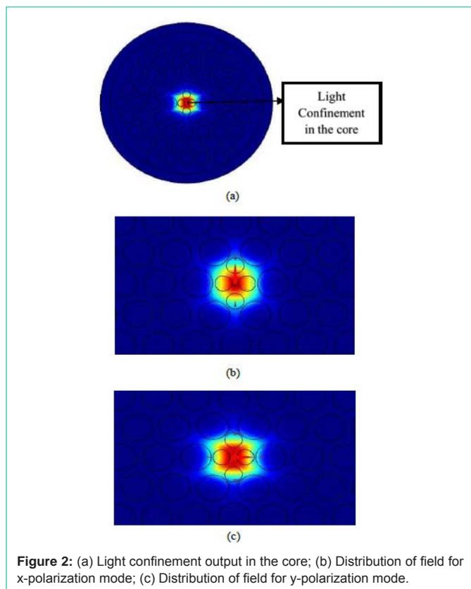
Figure 2: (a) Light confinement output in the core; (b) Distribution of field for x-polarization mode; (c) Distribution of field for y-polarization mode.
