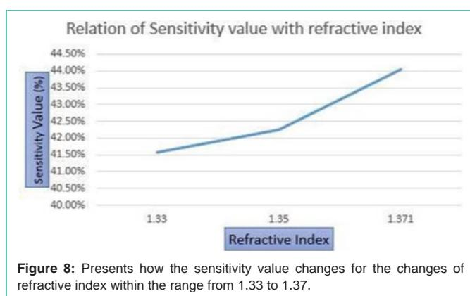
Figure 8: Presents how the sensitivity value changes for the changes of refractive index within the range from 1.33 to 1.37.
