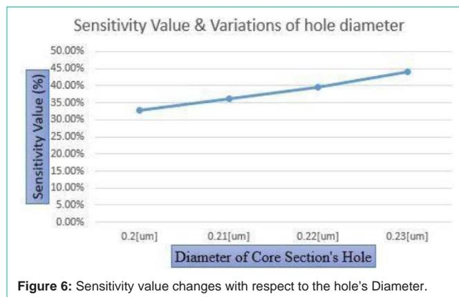
Figure 6: Sensitivity value changes with respect to the hole's Diameter.
