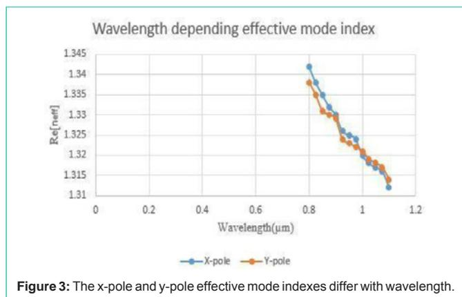
Figure 3: The x-pole and y-pole effective mode indexes differ with wavelength.
